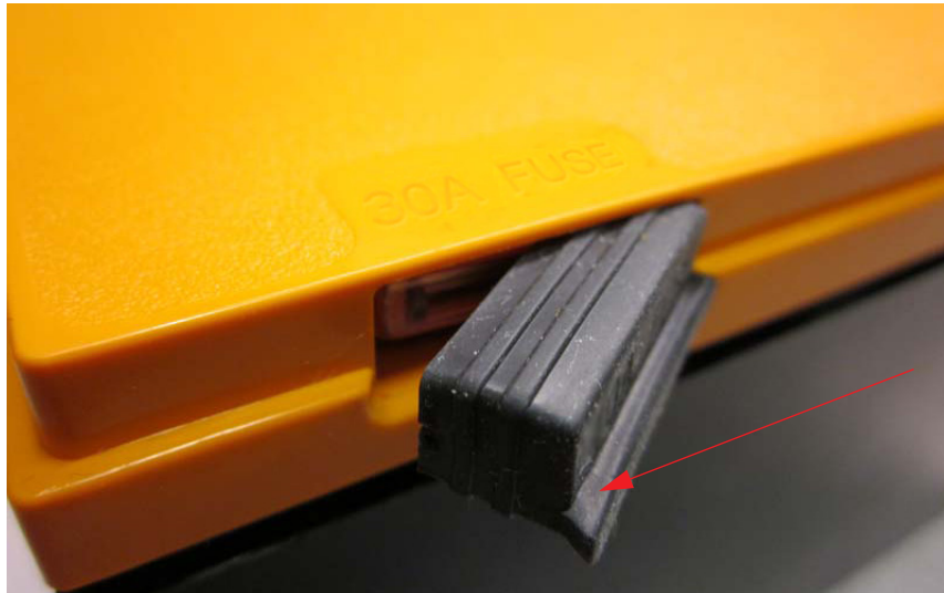
Figure 5-6 Removing the Fuse Plug
